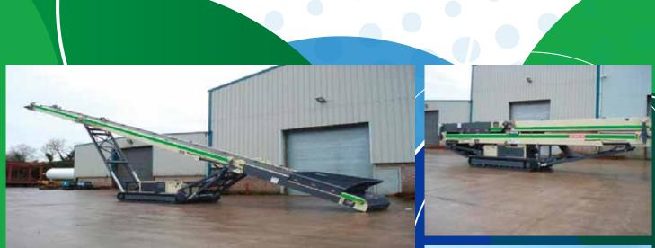
A leading manufacturer of screening and conveyor equipment, offers the MC1050-24T tracked stacking conveyor, the ideal solution for jobs that require high production stockpiling or material transfer.
